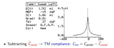
• At 226 Hz, estimate the residual canal compliance  $\hat{C}_{canal}$
