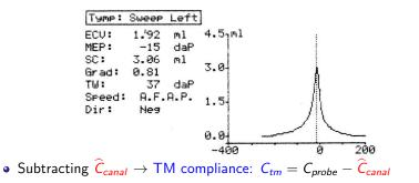
The key objective is to measure SC: the volume of the TM
