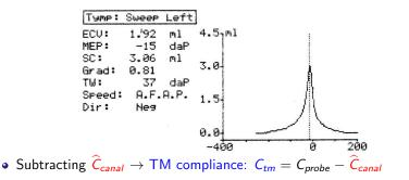
The key objective is to measure SC: the volume of the TM
