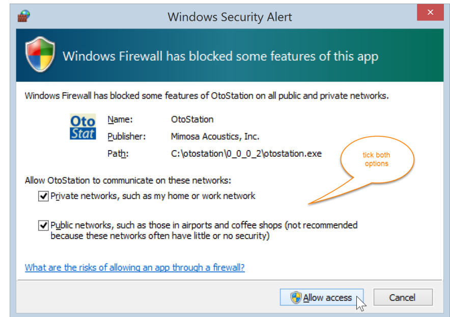
Figure 2.2: Allow your firewall Public and Private access to OtoStation. This example shows Windows Firewall. Your firewall may look different but still should offer similar settings.
