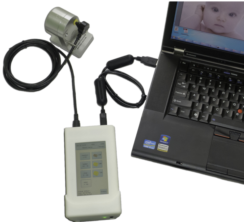
Figure 1.4: The OtoStat System connected to the support computer. The probe is mounted into the calibration cavity set. (The power adapter cable is not shown).
