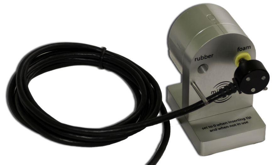
Figure 4.1: Probe with foam eartip mounted into the calibration cavity set (calibrator), which is set to Position 0.
