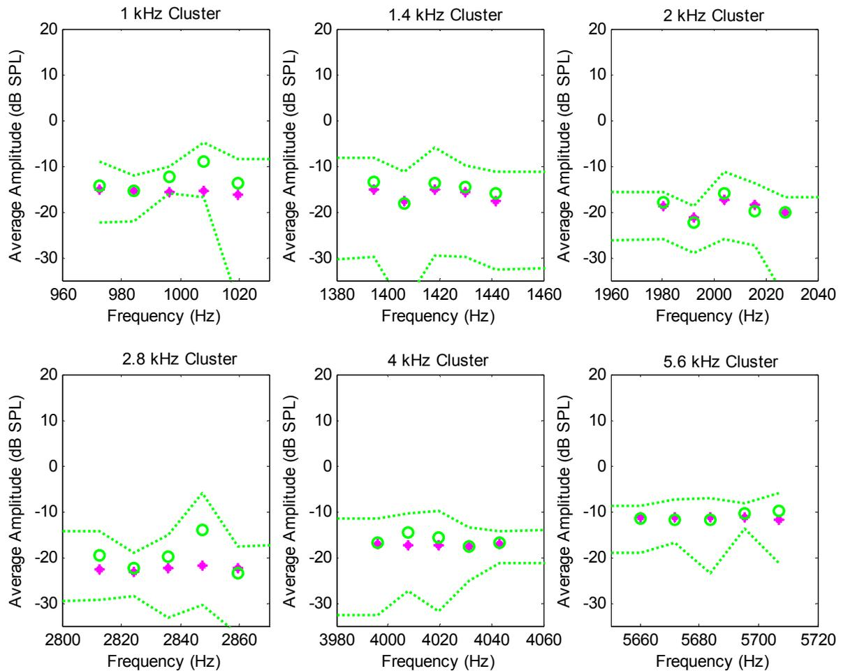
Figure 2 Average amplitude of SFOAE measurement and associated noise level in hearing-impaired ears ( $N=7$ ) for each frequency cluster. Only measurements with stimulus levels on target and low noise levels were included. Green circles are “SFOAE” responses, magenta asterixes are total noise level. Dotted lines indicate the averaged maximum and minimum responses.
