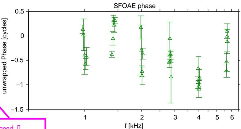
Calibration is not good. Channels are separated and spectrum is far from flat and smooth. Jitter indicates noise.
